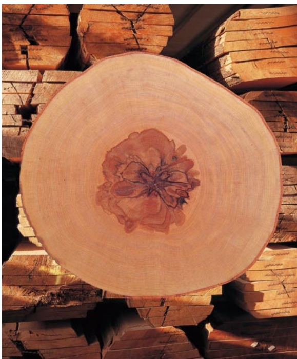
The red heartwood of beech trees is no longer a flaw, it is an eye-catcher.
